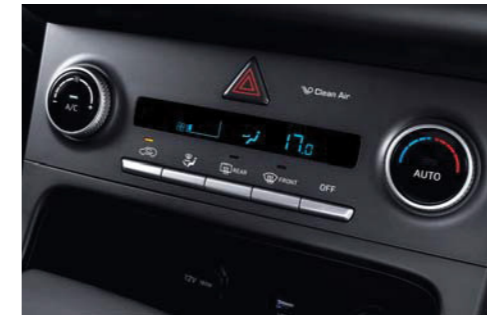
Full automatic temperature controls
