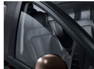
1st-row double-laminated soundproof glass
