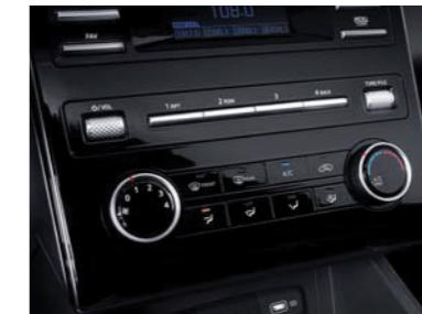
Manual air conditioning system
